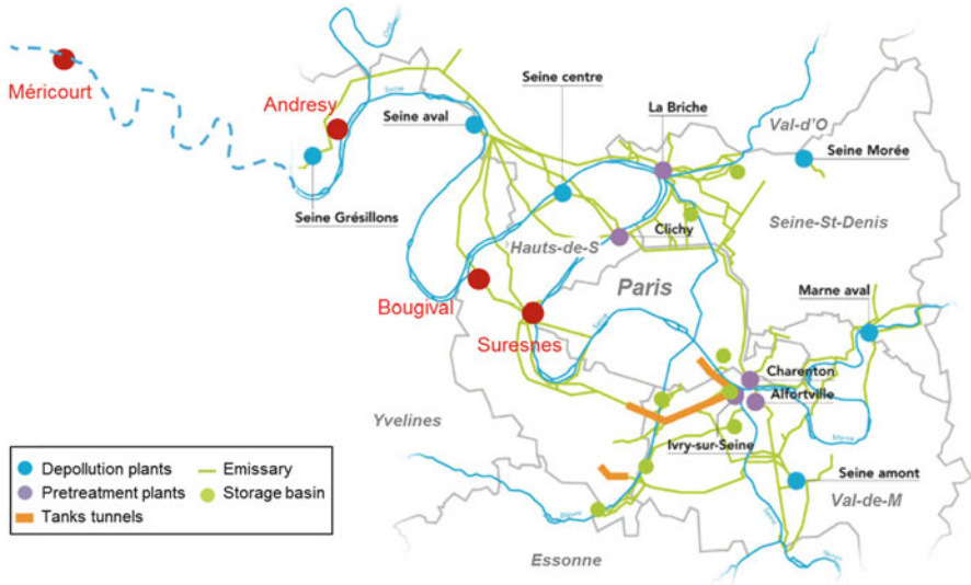
Fig. 2 Map of the Parisian conurbation indicating the WWTPs (blue circles and names in black, Seine Aval [SAV] previously Achères), the pretreatment plants (purple) and the storage tunnels/basins (orange and green), as provided by SIAAP. The four high-frequency O 2 monitoring stations are also indicated (red). Paris and conurbation départements (grey)
